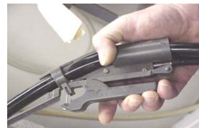
18. For units with remote bucket fill activation, hold and depress lever of remote gun. To stop flow, release lever. The lever can be locked on by flipping clip to hold lever. CAUTION: LEVER MUST BE MANUALLY UNLOCKED TO STOP FLOW. OVERFLOW WILL RESULT IF LEFT LOCKED IN OPEN POSITION.
